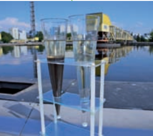
Settling test of activated sludge
